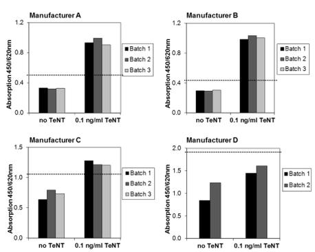
**Cutoff-based detection of TeNT in tetanus toxoids.** Toxoid batches from 4 vaccine manufacturers were tested in the BINACLE assay in pure form and spiked with 0.1 ng/ml TeNT. Shown is the mean absorbance from a 3-fold measurement of each sample. Dotted lines represent the cutoffs (mean absorption of the non-spiked batches plus 3-fold residual standard deviation).
