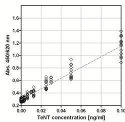
**Determination of the detection limit.** Dilution series of pure TeNT were tested in three BINACLE assays. Each sample was measured sixfold per assay. Shown are the raw data from all three assays and the resulting regression line (slope: 8.58, R-square: 0.945).
