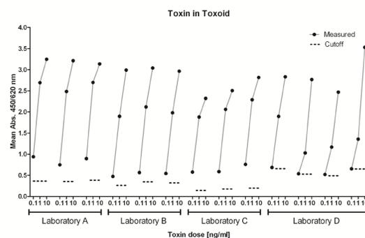
**Cutoff-based approach for detection of TeNT.** Each curve represents the mean absorption values obtained in one test with the TeNT concentrations indicated on the x-axis (0.1, 1, and 10 ng/ml) diluted in toxoid. The short dotted lines represent the corresponding cutoffs (mean absorption of the blank sample + 3-fold standard deviation) for each test.
